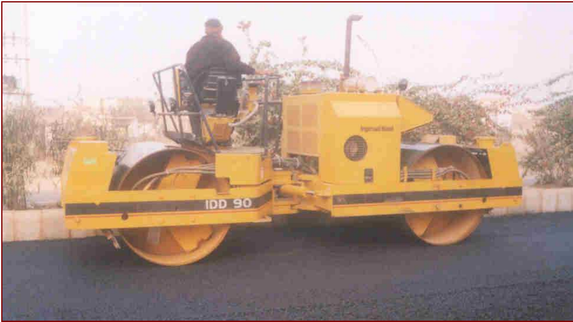
Tandem vibratory roller
